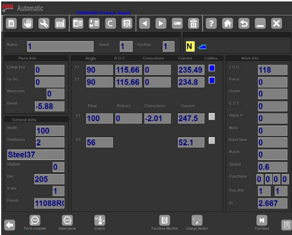
Figure 40 Double size automatic numeric mask as in the Kvara S 860 and S 660W PC models
