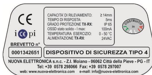
Fig. 12.5 Rear identification plate of RX
