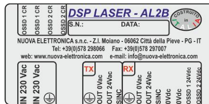
Fig. 12.9 Identification plate of AL2B module
